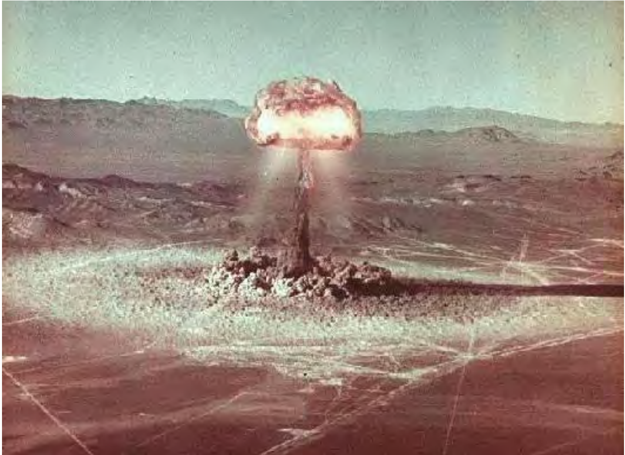
Figure 2-1. Photograph of Shot EASY in Operation BUSTER-JANGLE (AFLML, 1951) showing region closest to ground zero where thermal pulse had an important effect on resuspension of surface soil and blast-wave region extending beyond region impacted by thermal pulse where height of resuspended dust cloud was lower.
